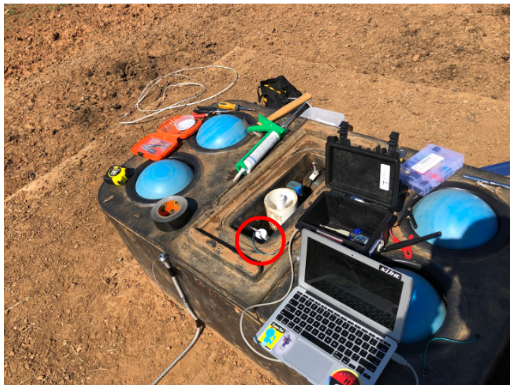
Figure 11: The compartment of the water trough that was removed to place the water level sensor within it as shown with a red circle.
