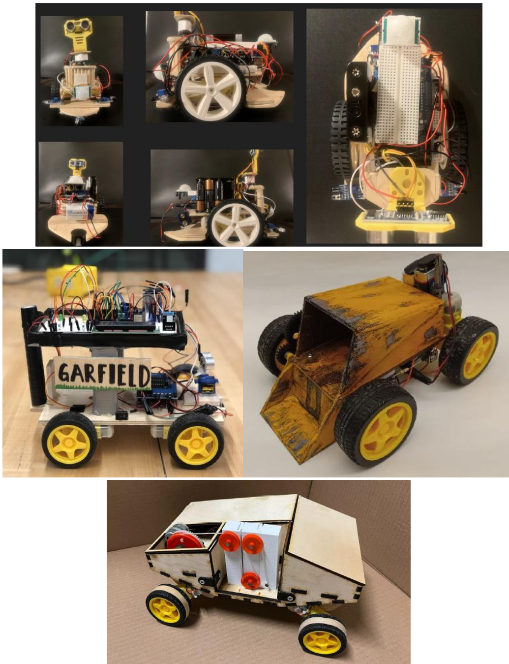
Fig. 1. Examples of design prototypes for the Mars in the Making project (top example: an astronaut companion robot; middle left example: a greenhouse assistant robot; middle right example: a rover to detect and harvest ice; bottom example: a rover to explore and document findings using images)
