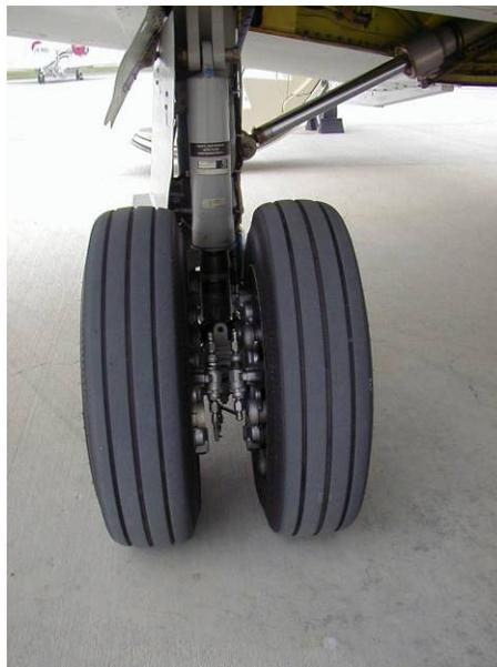
**Fig. 12a Disk Brakes for Citation VII Corporate Jet**
