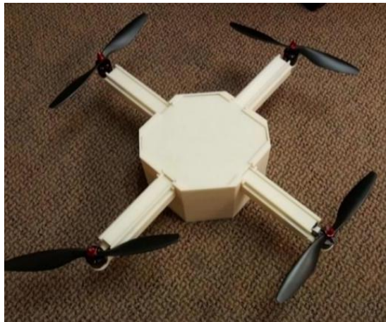
Figure 2: Picture of the current version of the drone developed by the students. The drone weighs 5.8 lb and has overall dimensions-including the arms- of 14x14in
