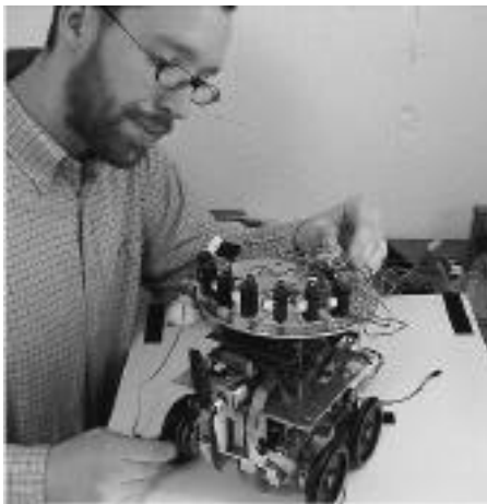
Figure 2. Trinity RST Student Building MiniBob's Sensor Array
