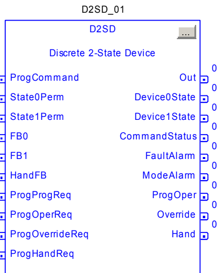
Figure 5 (Discrete 2-State Device)
