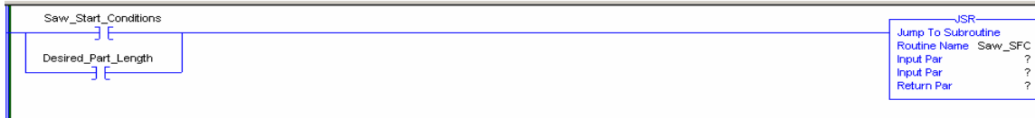
Figure 7 (New Saw Code in Ladder Logic as Programmed in RSLogix5000)
