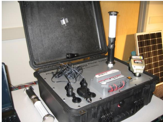
Figure 3 The photo of the PV emergency power system
