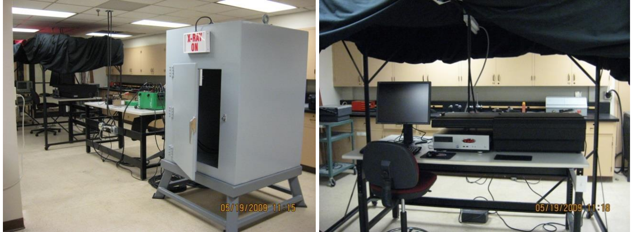
Figure 1. X-Ray tube/cabinet (left) & VMI laser scanner with image processing software (right)
