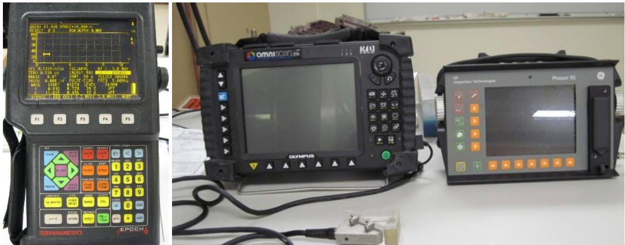
Figure 2. Olympus Epoch ultrasonic flow detector (left), Olympus Omniscan MX phased array ultrasonic flow detector (center) & GE Phasor XS phased array ultrasonic flow detector (right)
