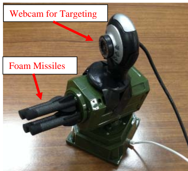
Figure 1. Auto-Targeting Turret Project using the Thunder Missile Launcher (with foam missiles) [7] and a Tecknet webcam [8].
