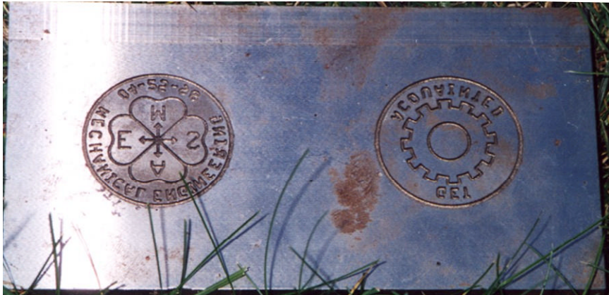
Figure 1. Die plate for stamping College of Engineering Open House Commemorative Coin
