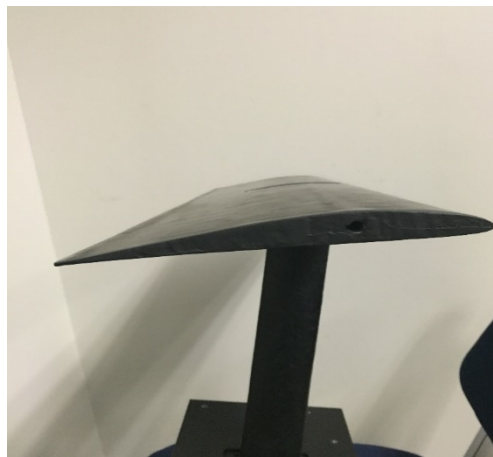
Figure 3. Eppler 387 on Test Stand
