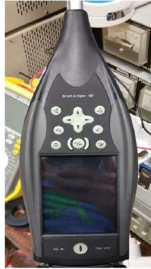
Figure 2. Brüel & Kjær ¼" Microphone and G-4 2270 Frequency Analyzer
