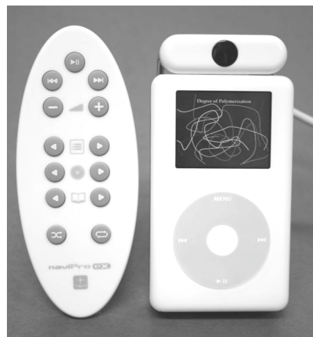
Figure 4: The iPod screen shows a PP slide from a polymers lecture. The remote control unit fits comfortably in a palm, and is handy for changing slides while standing away from the iPod.
