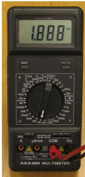
Figure 5. Maximum Segments Active for 3½ Digit DMM
