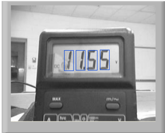
Figure 8. Webcam Image of DMM with Digit ROIs selected
