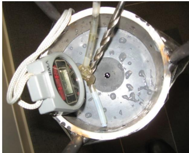
Figure 1. First Iteration of the Sharp-edged Orifice Demonstration [4]
