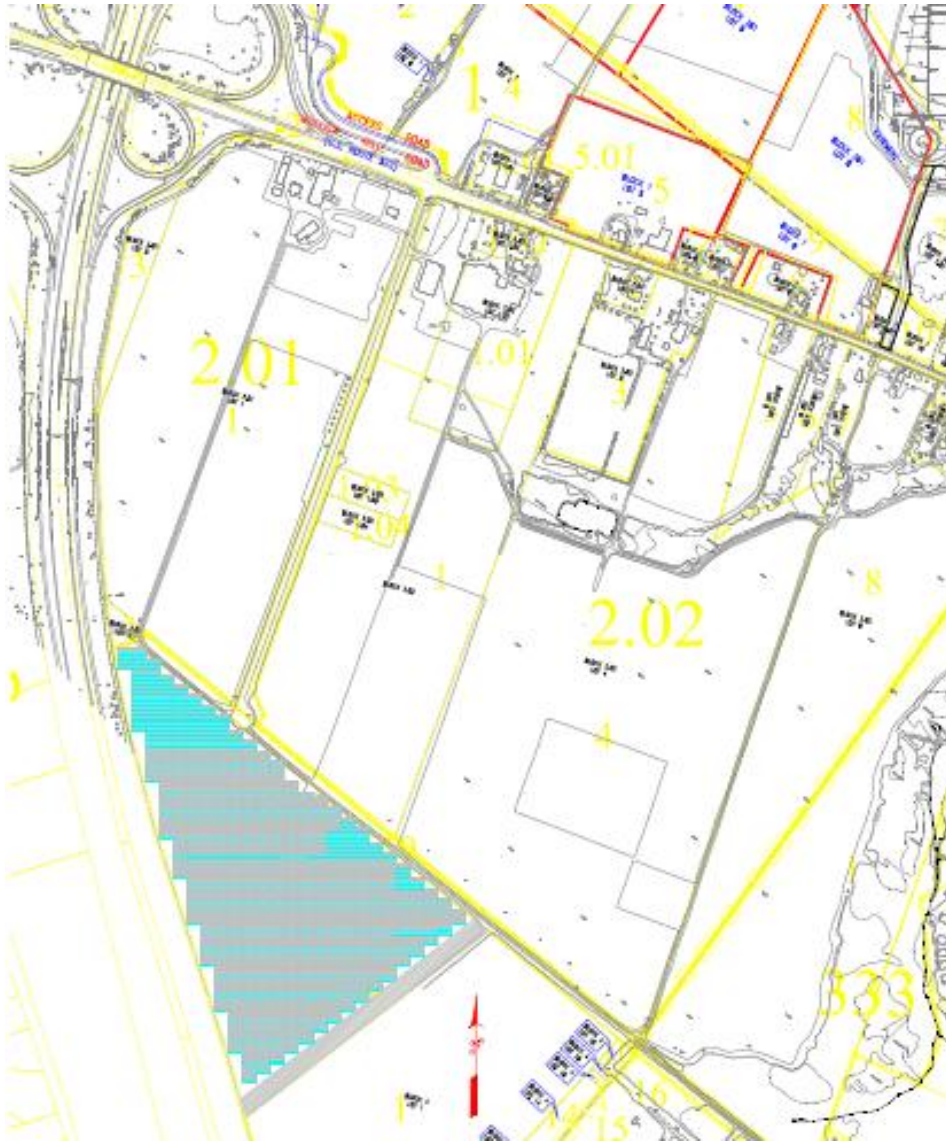
Figure 1. Site map of West Campus with preliminary design shown in the bottom left corner. Blue representing the PV modules, and Grey representing the expected inter-row shading.
