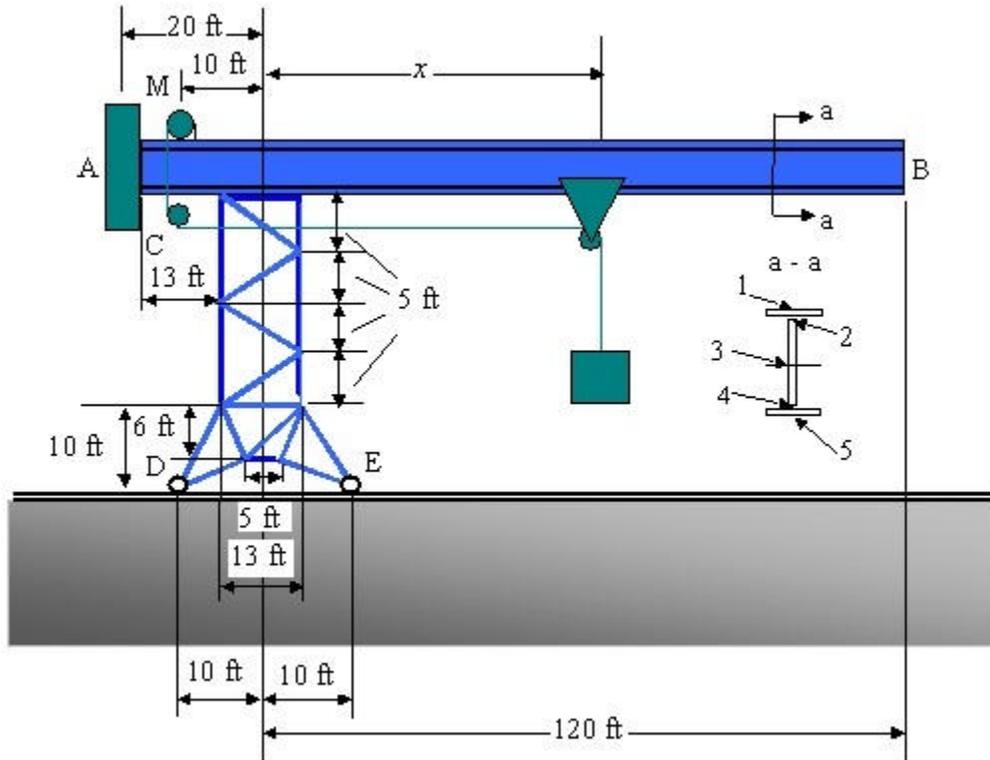
Figure 2: Schematic configuration of simplified tower-crane design
