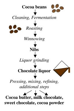
Figure 1: Overview of chocolate manufacturing process (adapted)[5].
