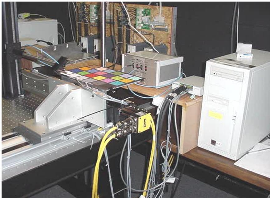
**Figure 1.** Typical layout for a Machine Vision workstation
