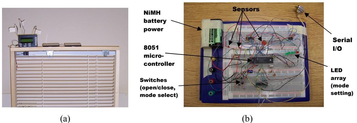
Figure 2. Prototype window with automatic blinds system. (a) Blinds assembly. (b) Microcontroller circuit.
