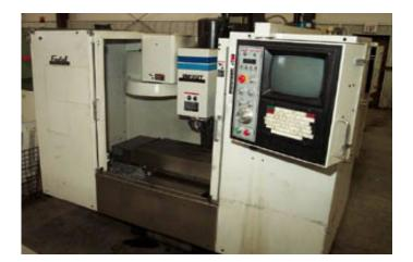
Fig. 2 A CNC machining center
