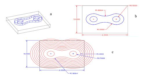
Fig. 3 a. A solid model of the part, b. a working drawing c. tool path
