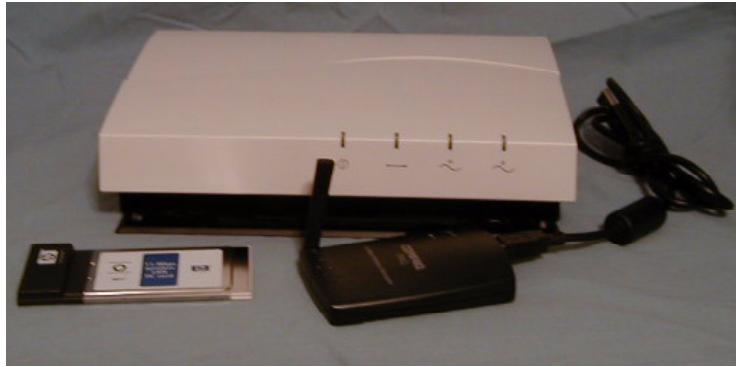
Figure 2. Wireless access point, external USB wireless network card, and laptop PC wireless card for a wireless network (clockwise from top)
