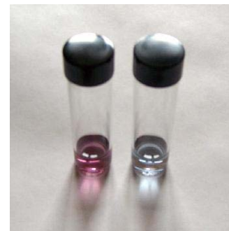
Figure 7. Colloidal gold solution before (left) and after (right) filtration through the microfluidic device.
