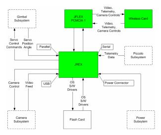
Figure 2 – UAV System Top-Level Block Diagram<sup>4</sup>
