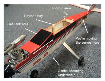
Figure 4 – Hardware Layout <sup>4</sup>
