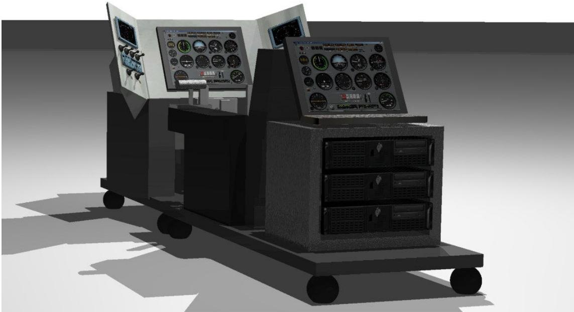
**Figure 13. Mobile Flight Simulator Early Concept Rendering without façade.**
