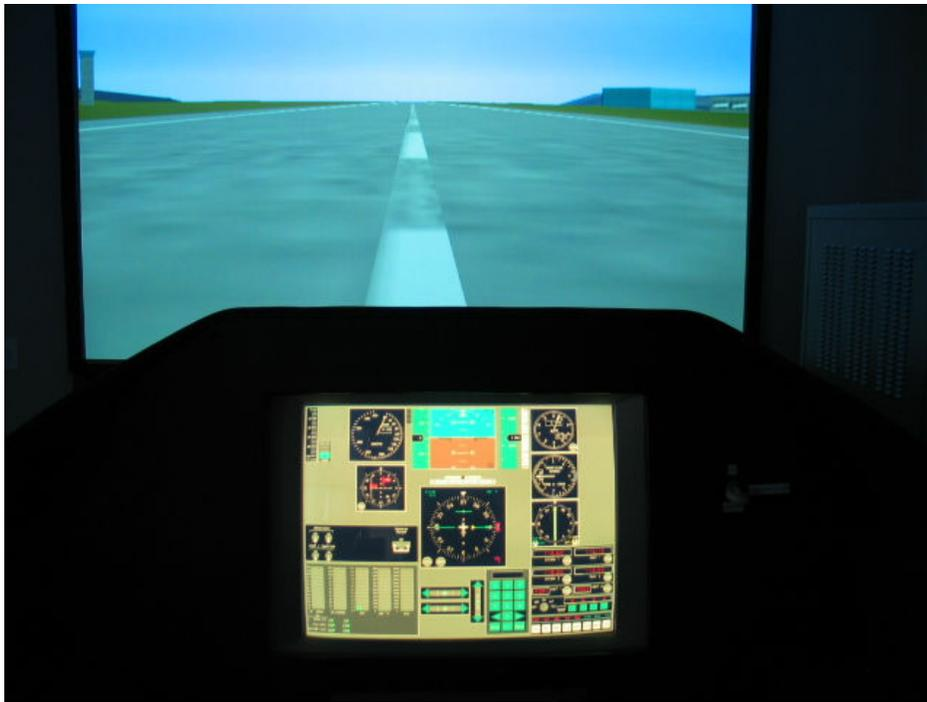
Figure 2. EFS Instrument Panel and out-the-window visual scene with lab darkened.
