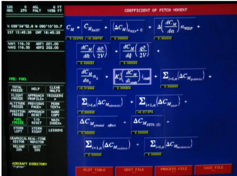
Figure 4. Pitching Moment Aero Model Development page on EFS IOS.
