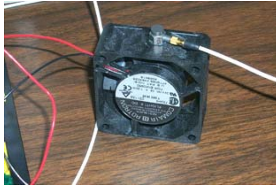
Figure 2: Motor accelerometer set-up.
