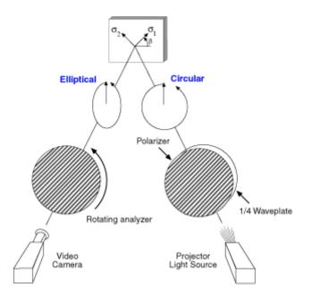
Figure 6.Grey-field Polariscope System Components<sup>10</sup>
