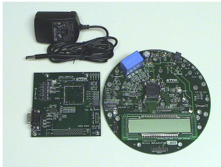
**Figure 1. TDK Demo and Debugging Boards.**
