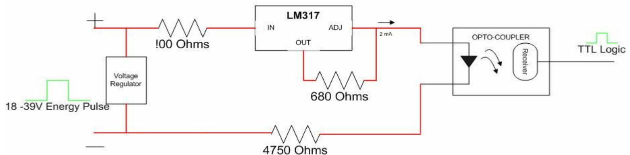
**Figure 4. Energy Pulse Circuit.**
