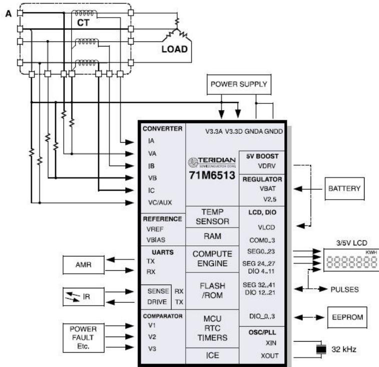
reference and 32 bit computation engine supports a wide range of polyphase metering applications with very few low cost external components. A 32 kHz crystal time base for the entire system and internal battery backup support for RAM and RTC further reduce system cost.
