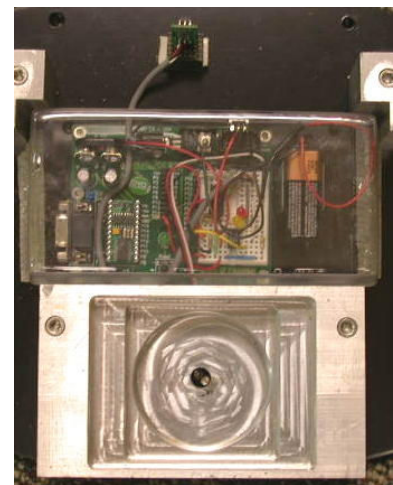
Figure 1: Smart Pallet - IR emitter/detector (top) - microcontroller (middle) - Cup holder (bottom)
