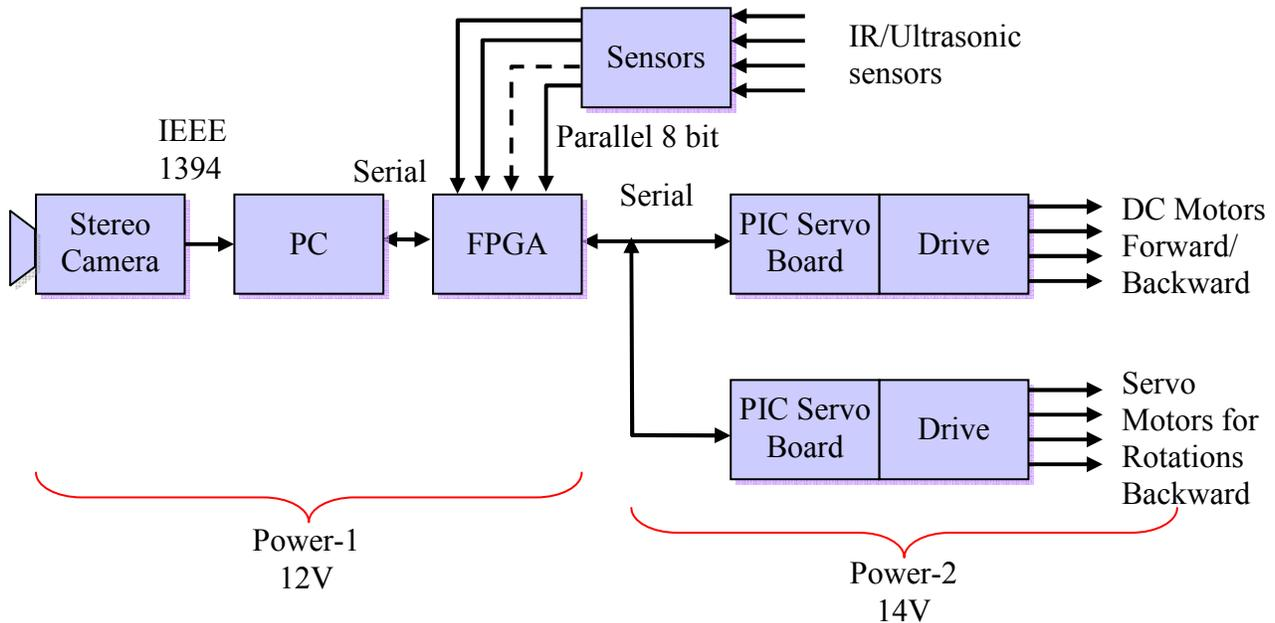
Figure 2. System diagram of A Smart rover with Stereo Vision
