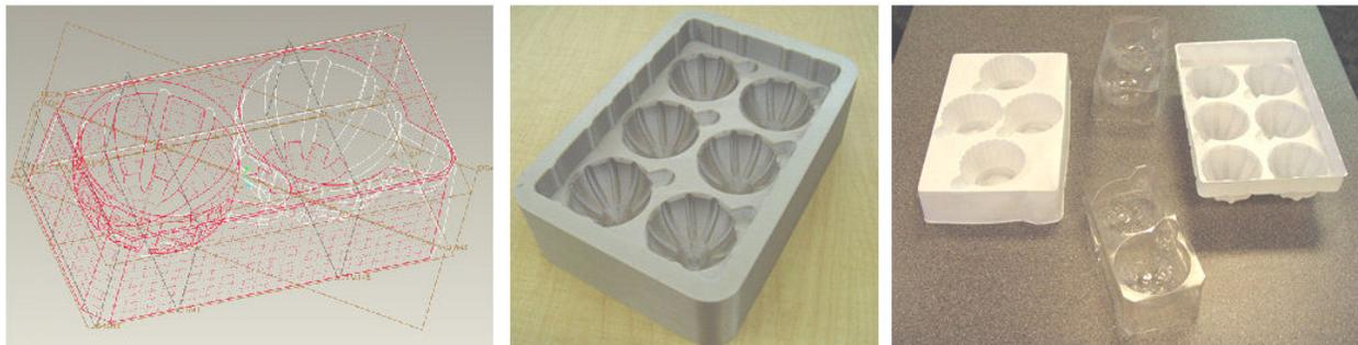
Figure 2: Ornament Trays: CAD model, mold, finished product
