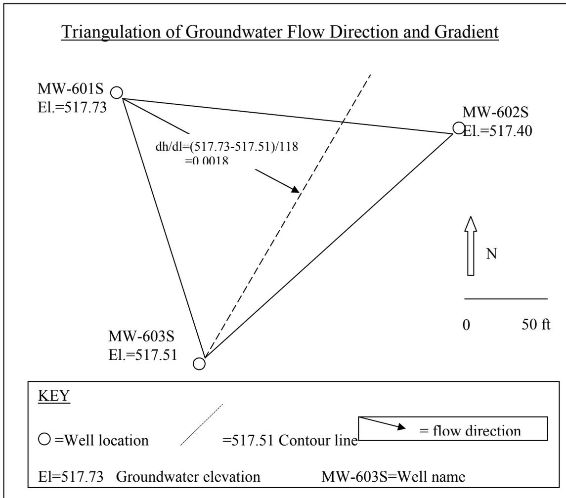
Figure 3. Triangulation of groundwater flow direction and gradient (Adapted from Hoffner<sup>5</sup>)
