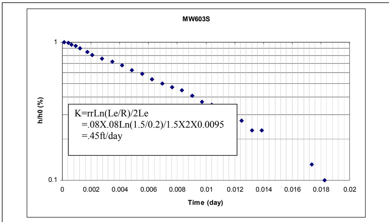
Figure 2, Data, h/h<sub>0</sub>, Vs. time graph and Hvorslev calculation for K, (Hoffner<sup>5</sup>)
