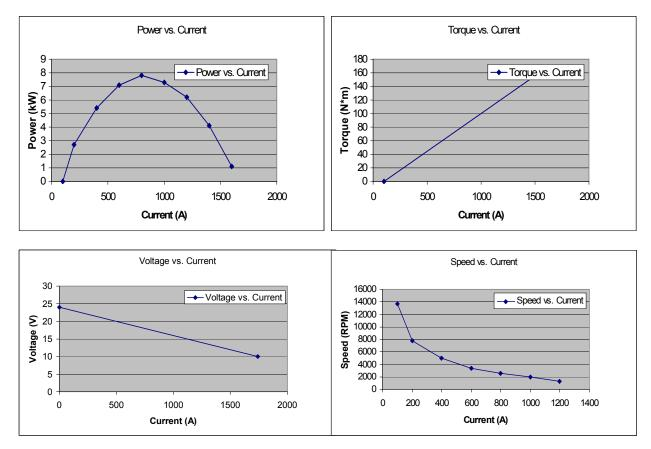
Figure 3. Electric Power, Torque, Voltage, Current, and Speed Characteristics for the motor
