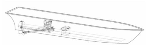
Figure 5. Drawing of eBoat with experimental pulley drive system
