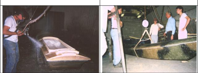
Figure 2. Fiber-glass Hull Manufacturing
