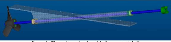
Figure 6. Three -dimensional model of new output shaft
