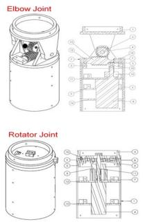
Figure 3: Low-cost manipulator joint design
