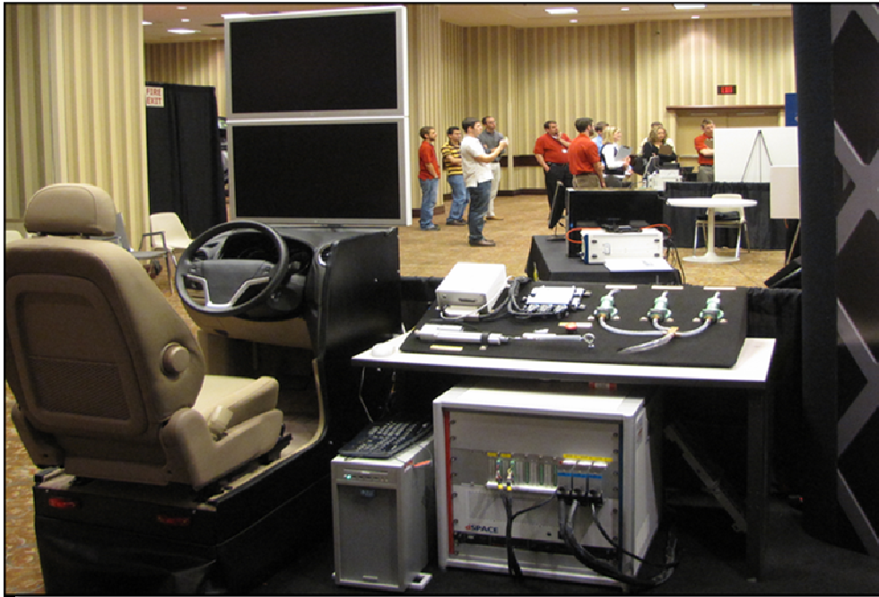
Fig. 3. A dSPACE hardware-in-the-loop configuration using their Microautobox and their simulator chassis
