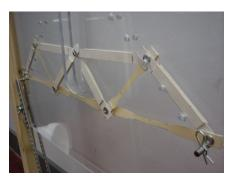
ultimate force that the truss can withstand.
