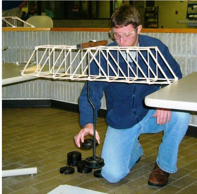
**Figure 1: Load Testing Apparatus**
