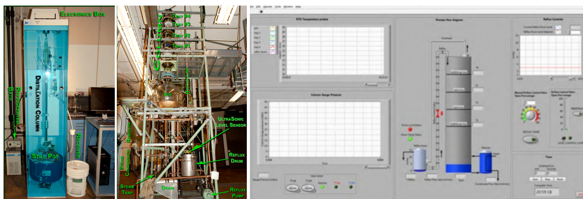
Figure 3: Images of the two distillation columns used in the laboratory (left) and an example of the new interface and online monitoring capabilities that have been added to them (right).
