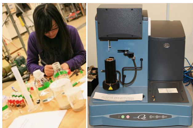
Figure 4: Student performing the jar-scale molecular sieve experiment (left). Image of the thermogravimetric analysis (TGA) equipment used in the desorption experiments (right).
