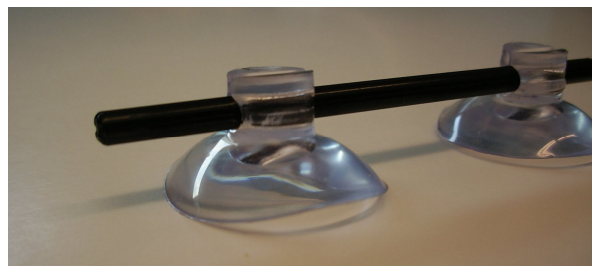
Figure 15 Suction cups attached to a Lego axle
