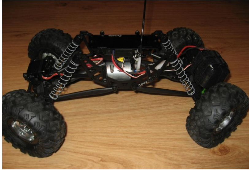
Figure 2: Raw Demo for Spring/Mass/Damper Lesson
