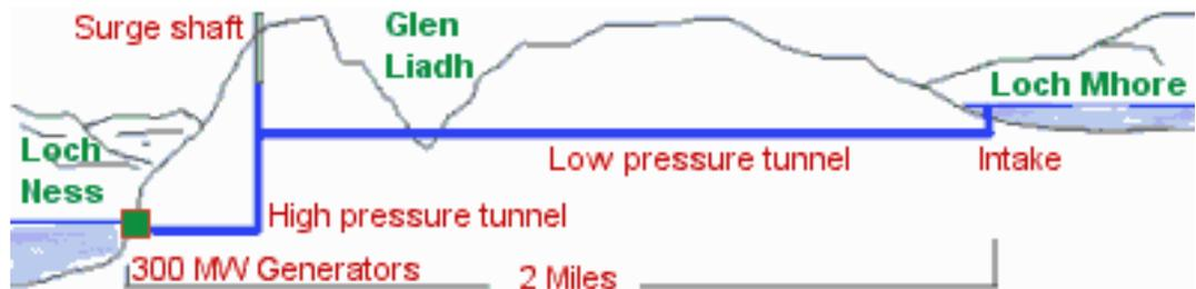
Figure 2. Schematic of FPHF [9, 10].
