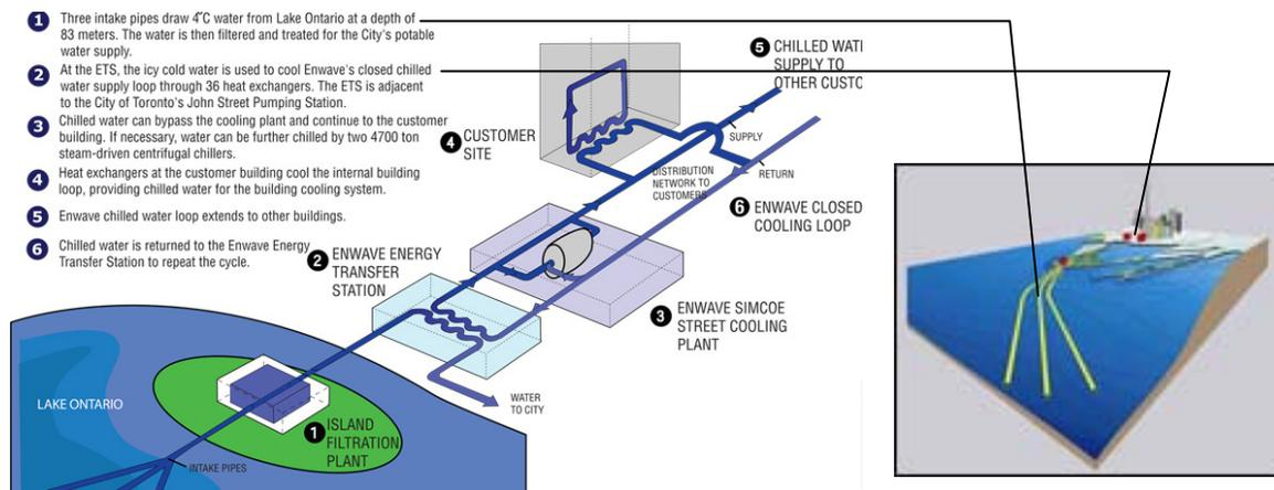
Figure 1. Deep Lake Water Cooling System Schematic [1, 2].
