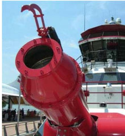
Figure 5. Fireboat Three-Forty-Three Primary Monitor (Nozzle) [14, 15, 19].
