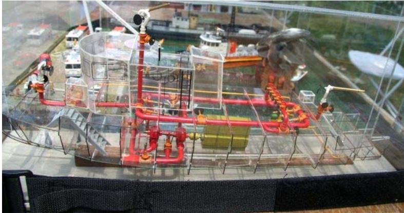
Figure 6. Cutaway Showing Piping for a Typical Fireboat [17].
