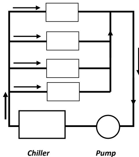
Figure E2. Z-layout schematic.
