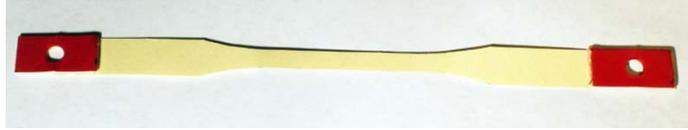
Figure 3. Actual test specimen with end stiffeners.
