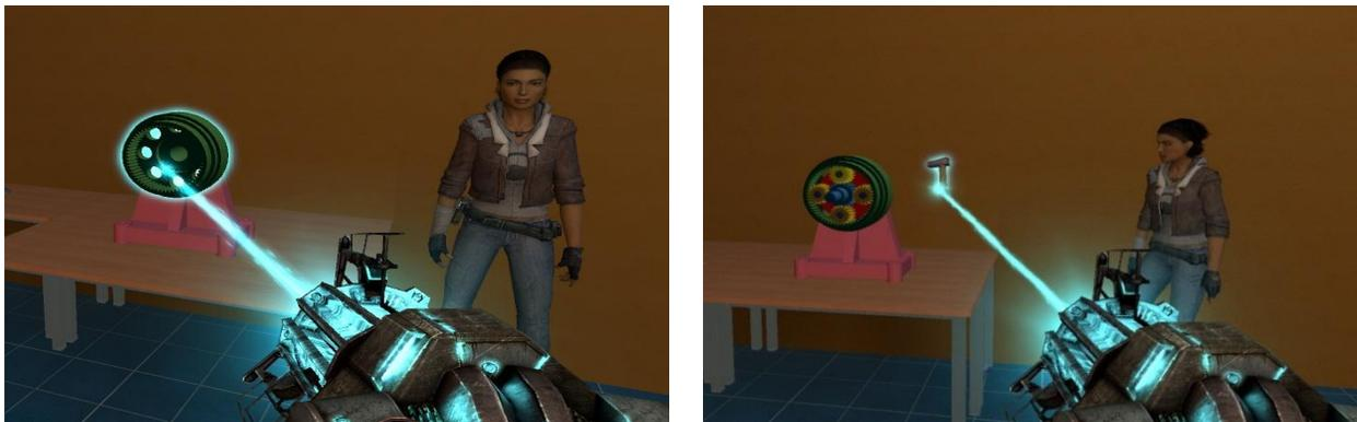
Figure 7: Assembly and disassembly operation in grabbing a ring gear by the 'physics gun' and mounting it on the base (left) and using a 'hammer' (disassembly tool) to signal a disassembly (right)
