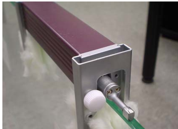
Figure 4: Stylus of the SJ-301 for surface roughness measurement on glass edge.
