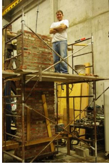
Master's student Dan Lazzarini tests a post-tensioned masonry wall as part of his project
