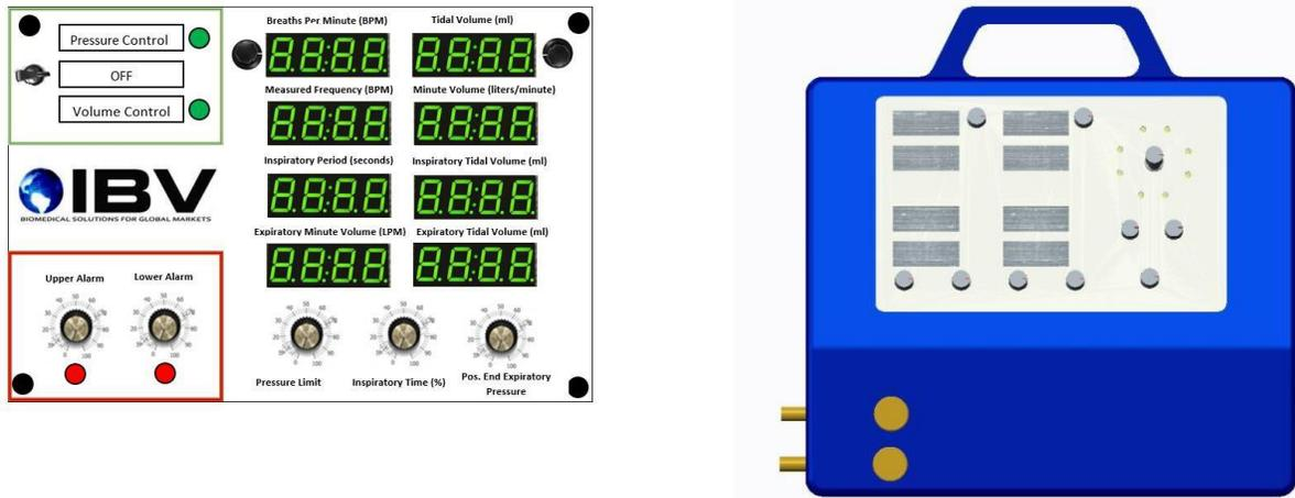
Fig.1.6 Schematic of the Ventilator
