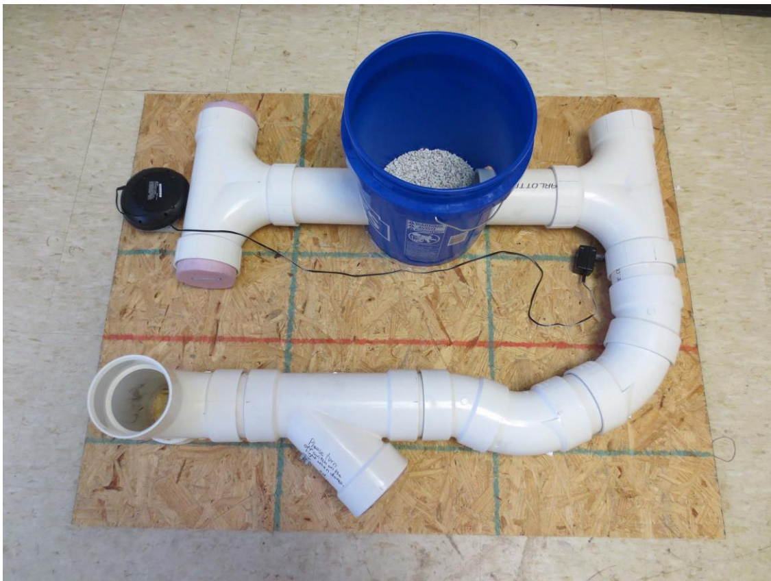
Figure 6. Top view of final project maze. Entry point is on the bottom left of the image. The light switch is in the first lateral at the bottom of image. A ball obstructs the path before the first tee on the right. The bucket is filled with loose gravel. A digital clock is placed at the left, and the metal ball bearing is on a ledge inside the final tee.
