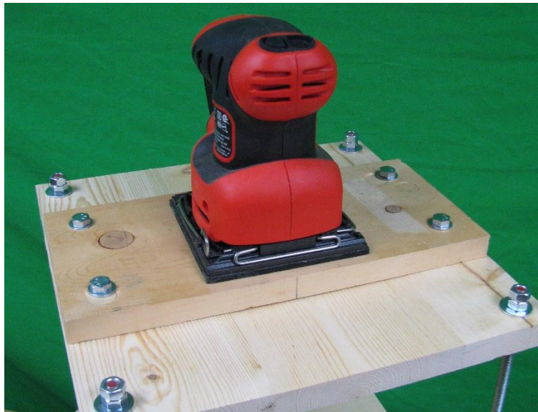
Figure 5: Mounting of the Orbital Sander Vibration Source
