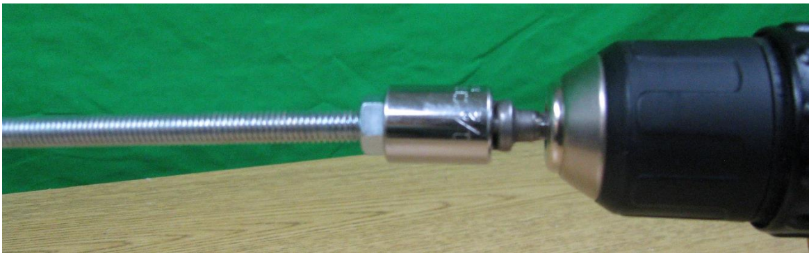
Figure 3: Use of the Jam Nut to Spin the Threaded Rod for Nut Placement
