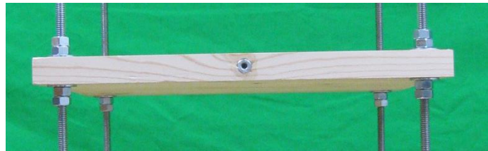
Figure 6: Mounting Nut for the Accelerometer
