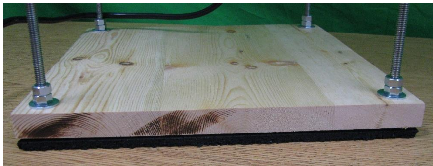
Figure 7: Damping Layer Underneath the Lower Tier
