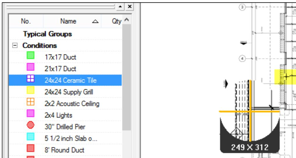
**Figure 3.** Area takeoff with grid example.
