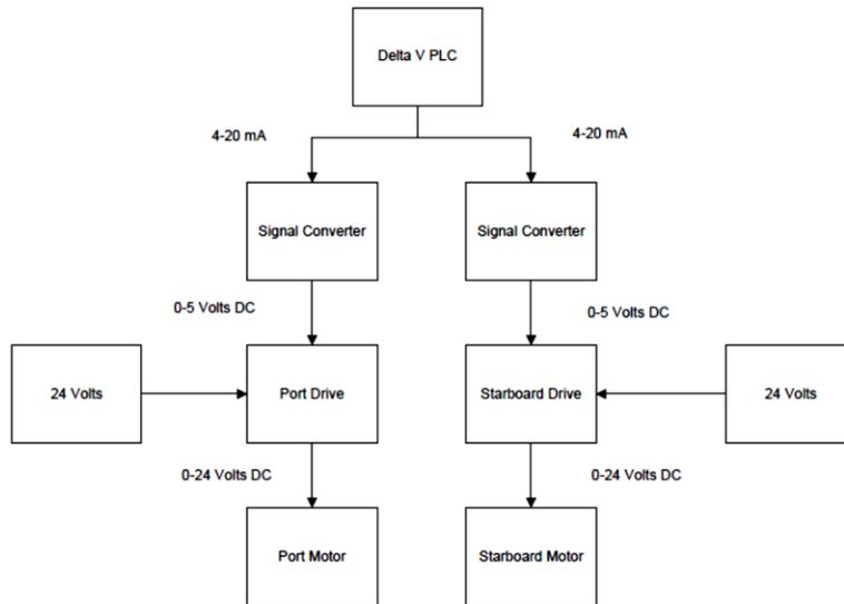
Figure 1 Block Diagram for SLIM Drive System
