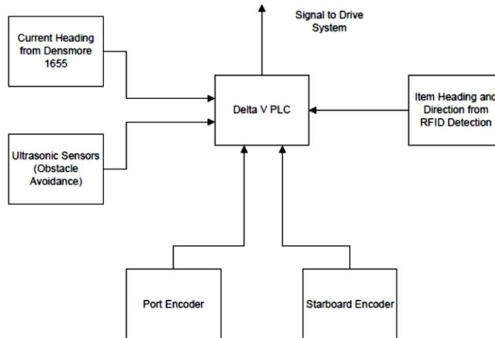
Figure 2 Navigation System Block Diagram
