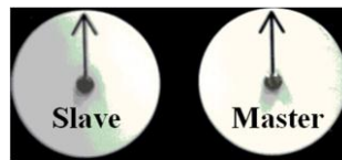
Fig.3: Two servomotors with arrows indicating the current phase of their shafts
